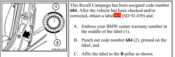
If the vehicle already has a label from a previous Service Action/Recall Campaign, affix the new label next to the old one. Do not affix one label on top of another one, because a number from an underlying label could appear in the punched-out hole of the new label.
