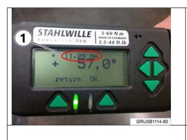
15. While performing the angle torque, the digital screen on the torque wrench will display the current Nm meter value. This value should be between **8 Nm-14 Nm**.
