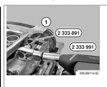
14. IMPORTANT: The bolts require initial torque and angle torque. Observe the procedures in this step and the next step very carefully!
